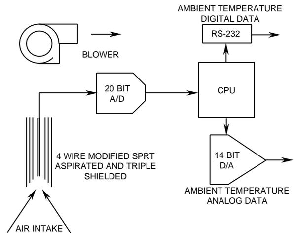
**PMT-2005 functional block diagram**
