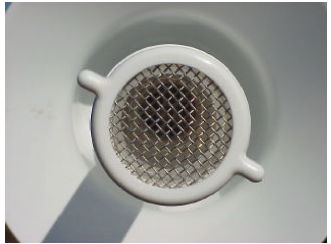
Detailed view of bottom of temperature sensor showing double intake radiation shields, canopy shade ring, and screen.
