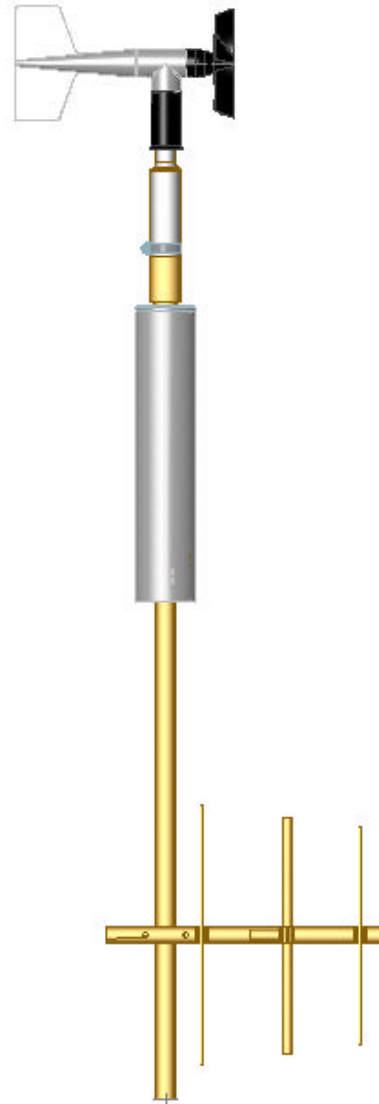
TMS-7200 Weather Sensor, (Yagi antenna below)
