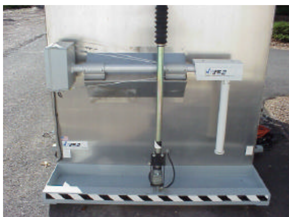
Thermohygrometer with pressure sensor mounted on back of MERV provides surface temperature, dew point, and barometric pressure.
